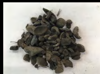
Palm kernel shell used in biomass power generation plant
