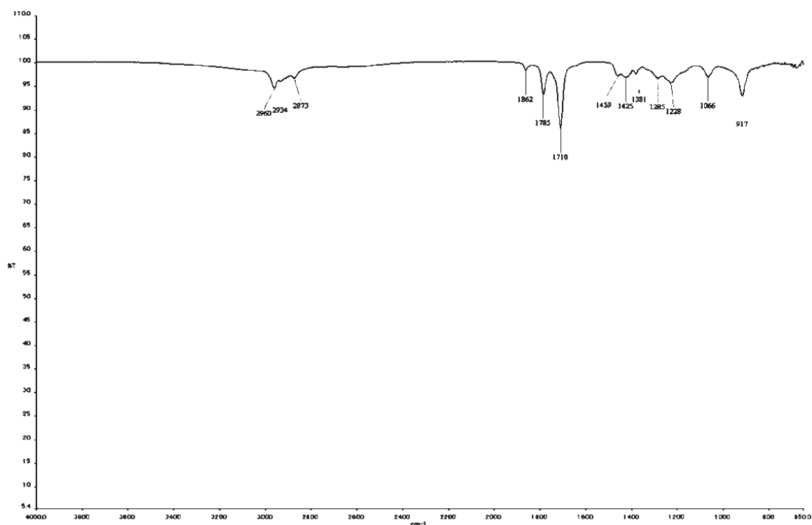
Figure 7-2 Experimental measured IR spectrum of hydrated tetrapropenylsuccinic anhydride
