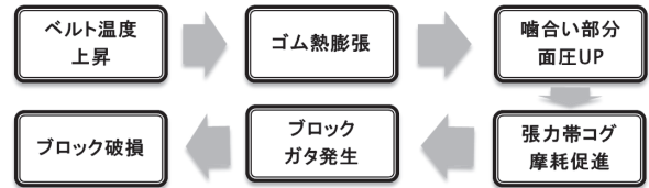
Figure 9 Belt fault mechanism at speed increasing ratio
